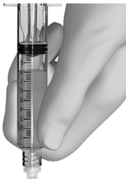
**i** *The plunger of the VPC must be dry, otherwise the pressure column will not be built up.*
