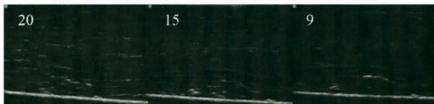
Fig. 6.20 Histogram values of a 13MHz linear probe without probe cover (left), with a glove as probe cover and two jelly layers (middle), and with a specific ultrasound probe cover with one jelly layer (right). The numbers indicate the specific histogram values from the entire screen shot (approx. 100,000 pixels for each screen shot).
